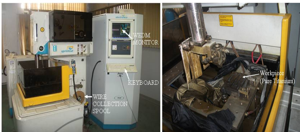
Fig.2. (a) Experimental Set up and (b) titanium workpiece machined with WEDM
